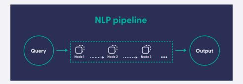
A basic pipeline consists of input and output modules, which are connected by one or more consecutive nodes. Other than that, there are no limits to creativity. Nodes can be added, removed, or swapped. Developers can even design parallel branches within the pipeline, or use multiple output nodes. The next section showcases a few pipeline designs.
